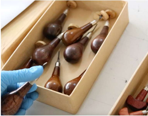
Figure 6. Burins used in engraving copper. Tools belong to the Printmaking Workshop from the Faculty of Fine Arts of the University of Porto. Photo by: David Lopes. 2022. Pure Print Archeology. (i2ADS/FBAUP).
