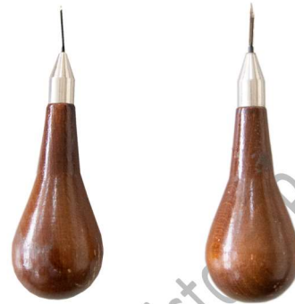
Figure 6. Burins used in engraving copper. Tools belong to the Printmaking Workshop from the Faculty of Fine Arts of the University of Porto. Photo by: David Lopes. 2022. Pure Print Archeology. (i2ADS/FBAUP).
